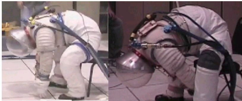
Figure 31: Pressurized I-suit Max Hip Flexion
