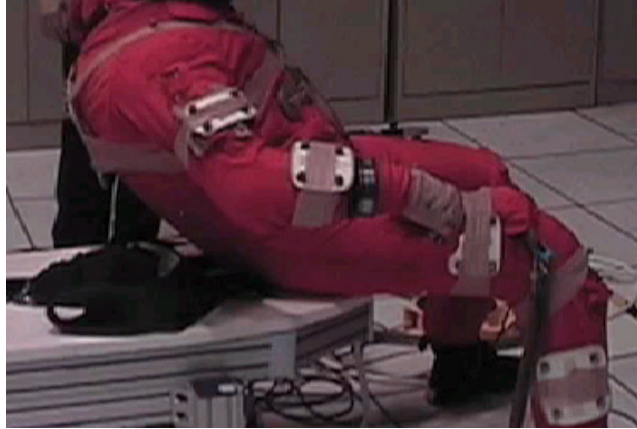
Figure 77: Pressurized ACES Elbow Bias
