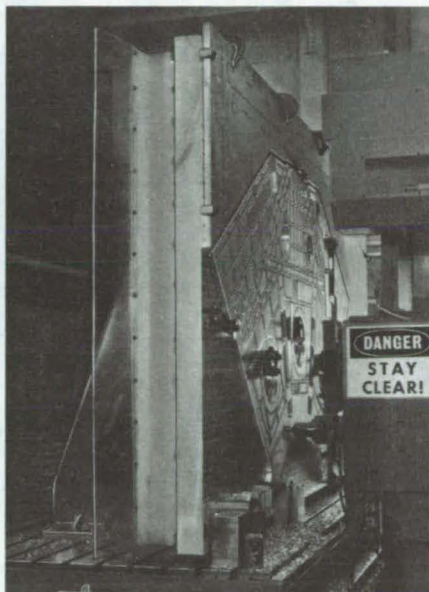
A Clear Plastic Shield is in position to intercept flying chips from a machine tool (left) and retracted to give the operator access to the workpiece (middle). The view from behind the platen (right) shows the hinge. Machine shops can readily make such shields for their own use.
