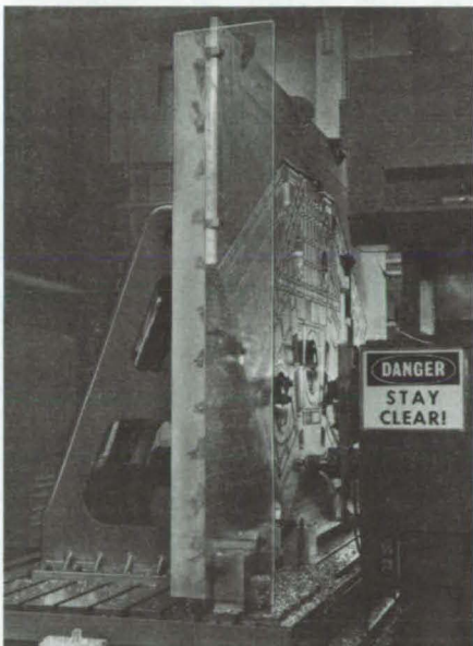
A Clear Plastic Shield is in position to intercept flying chips from a machine tool (left) and retracted to give the operator access to the workpiece (middle). The view from behind the platen (right) shows the hinge. Machine shops can readily make such shields for their own use.
