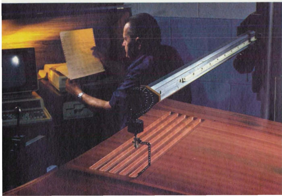
At left, a Visioneering engineer checks tolerances for an autohood model made from Ren epoxy resin model material. The new material was originally developed for modelling Space Shuttle thermal tiles. Above, Visioneering's numerically-controlled Duplex Milling Machine cuts model parts from Ren Shape boards. The Ren Shape line is attracting private sector interest as a replacement for traditional modeling materials used in automobile, aerospace and foundry industries.
