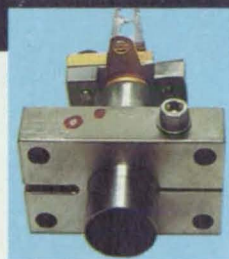
LED read station with optics.
