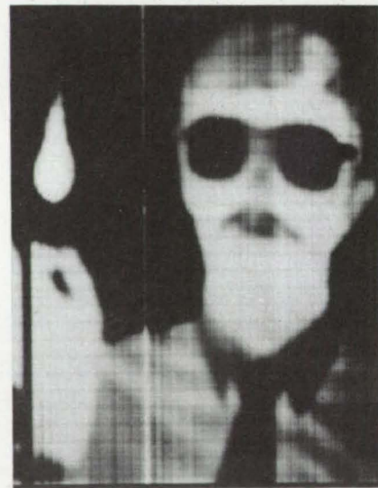
Figure 2. This Image of an Infrared Scene was generated by the photodiode array with the aid of a scanning mirror. Dark-current subtraction and computer processing would further improve image quality.
