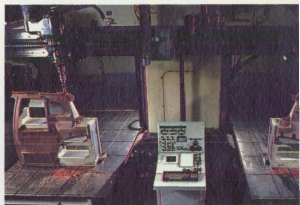
At left, a Visioneering engineer checks tolerances for an autohood model made from Ren epoxy resin model material. The new material was originally developed for modelling Space Shuttle thermal tiles. Above, Visioneering's numerically-controlled Duplex Milling Machine cuts model parts from Ren Shape boards. The Ren Shape line is attracting private sector interest as a replacement for traditional modeling materials used in automobile, aerospace and foundry industries.
