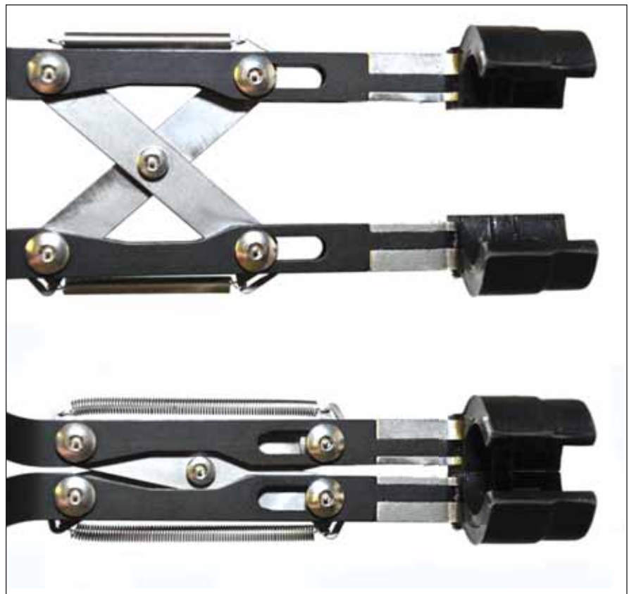
The Mate/Demate Pliers, shown in their open and closed configurations, feature cross-link springs to ensure they remain in the open position until adequate force is applied to close them.
