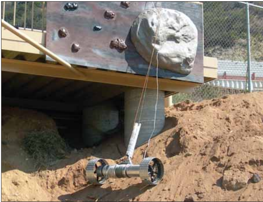
Figure 1. A Prototype Axel Rover can operate in a free or tethered configuration. Testing of this version is complicated by a need to properly wrap the power cable around the axle housing. It has been proposed to eliminate the power cable and install rechargeable batteries in a future version.
