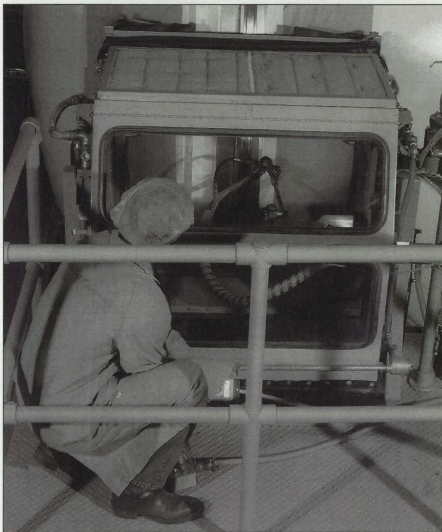
The Portable Spray Booth includes a contoured shroud and carbon filter bed that limit concentration of fumes in the vicinity.
