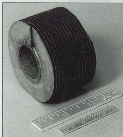
Figure 1. The Finned Aluminum Extrusion With Activated Carbon and Binder enables the effective transfer of heat from or to the sorbent as it adsorbs or desorbs a gas.
