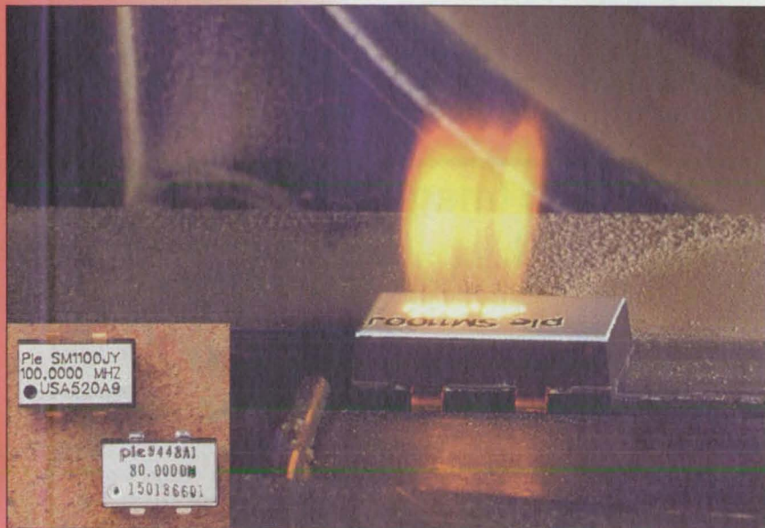
Inset: Comparison of print quality on ink-marked (lower) and laser-marked (upper) chips
