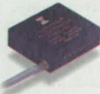
7290A Accelerometer. Ideal for low-level accelerations from 2g to 100g full scale. Offers dc response, ruggedness to 10,000g's, amplified ( \pm 2\text{V} ) output and a wide temperature range.
