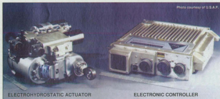
Figure 1. This Flight-Control Actuator comprising an electrohydrostatic actuator and electronic controller are used to operate the left aileron in the F/A-18 Systems Research Aircraft, without need for the usual central aircraft hydraulic system.
