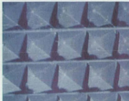
Ferrite Resin Cast With a Periodic Array of Pyramids Designed for a Frequency of 200 GHz
