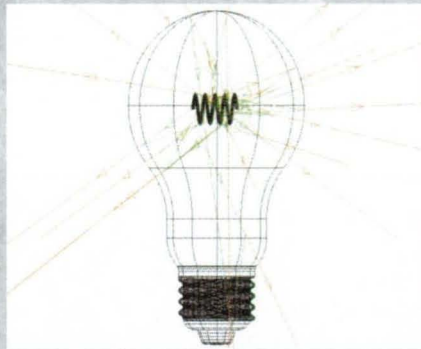
Complex objects may be imported, like this IGES light bulb. Other objects, such as this lenslet array, are generated within OptiCAD.
