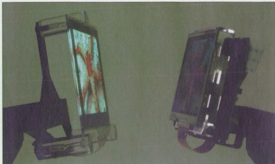
Figure 2. The active-matrix OLED display (left) as contrasted with a conventional LED display.
