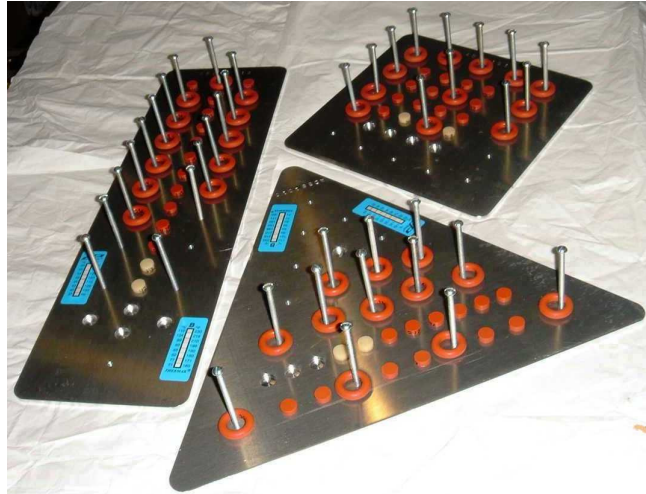
Figure 7.—Photograph of the specimens prior to bagging and electron radiation exposure; the square plate is 18.2 cm wide.
