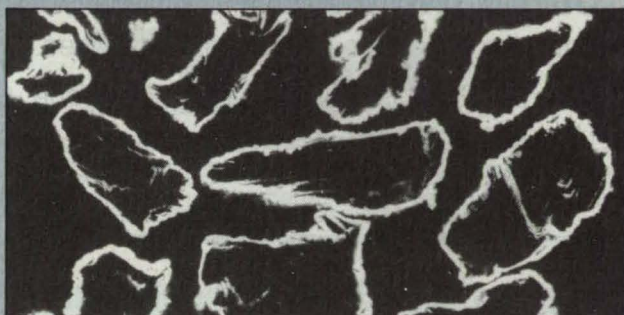
Novamet Nickel Coated Graphite, 60% fully encapsulated Ni, apparent density 1.6 g/cc, particle size (FSSS) 100 microns, screen mesh 63% - 150/+ 250, surface resistivity 0.3 \Omega/\square .
