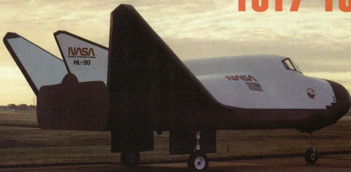
The HL-20 is Langley's candidate vehicle to complement the space shuttle, designed primarily for the transport of space station crews.
