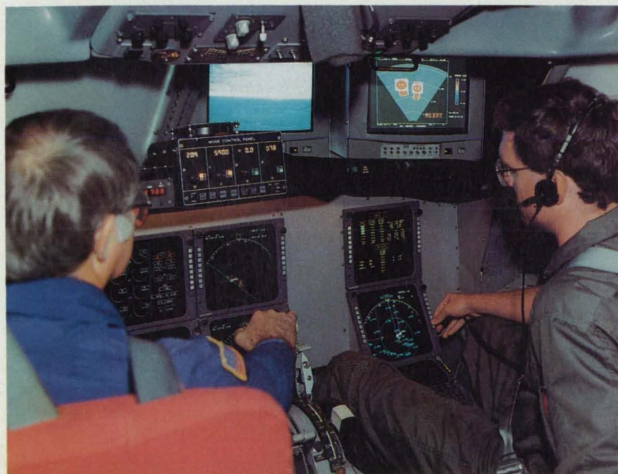
The cockpit of Langley's Transport Systems Research Vehicle displays data from an advanced-warning system for wind shear.
