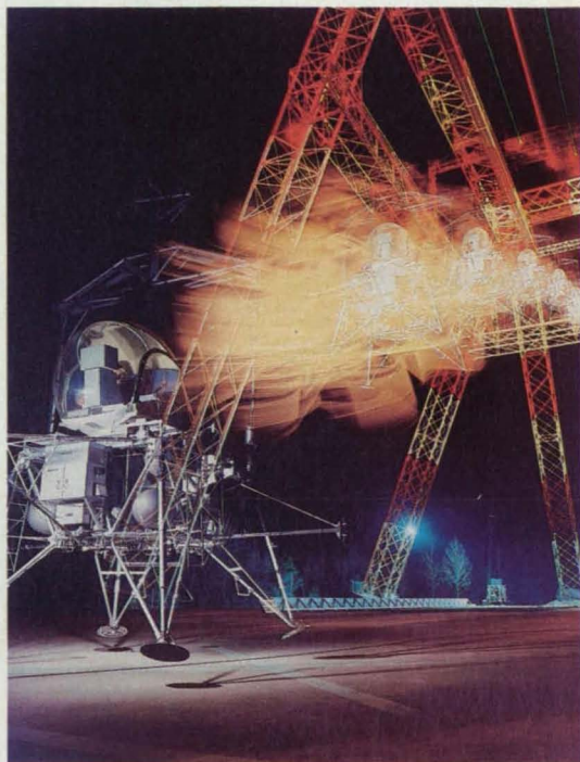
A multiple exposure captures the movement of the Lunar Excursion Module, a manned simulator designed by Langley to train Apollo astronauts.
