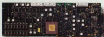
The DT3851: 1K x 1K input for high resolution devices.
