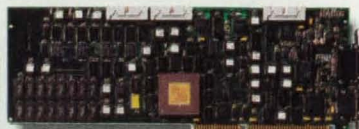
The DT3851: fast four-channel multiplexer for inspection with multiple cameras.
