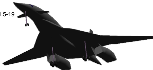
Figure A.1.5 072B Landing Gear Integration
