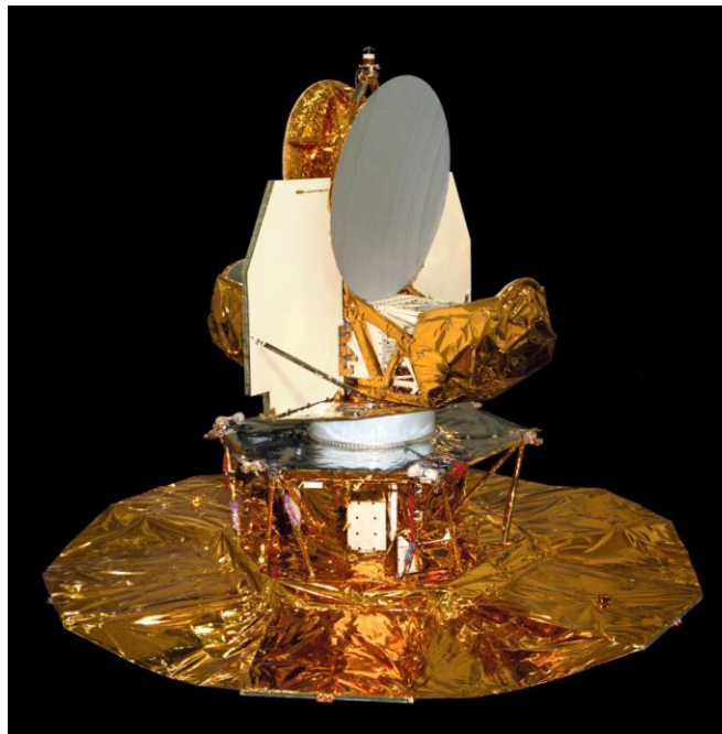
Figure 6.1-1. Spacecraft Overview - WMAP Observatory with Sunshade shown (bottom)
