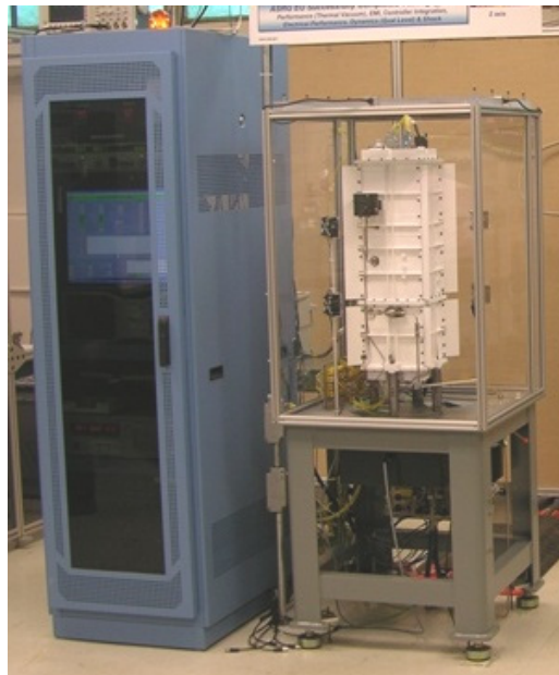
Figure 1.—ASRG EU test station. ASRG EU in an enclosure on test stand inside the ASRG EU and ASC-E #1 and #4 special test facility.
