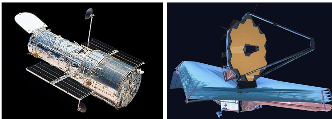
Figure 5. The Hubble Space Telescope LEO on-orbit configuration (left) versus that of the James Webb Space Telescope in its L2 orbit (right)
