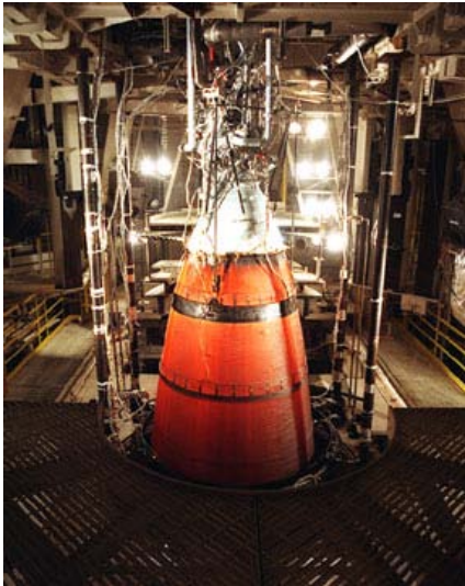
Figure 36. The RL 10B-2 Engine in J-4 Test Cell
