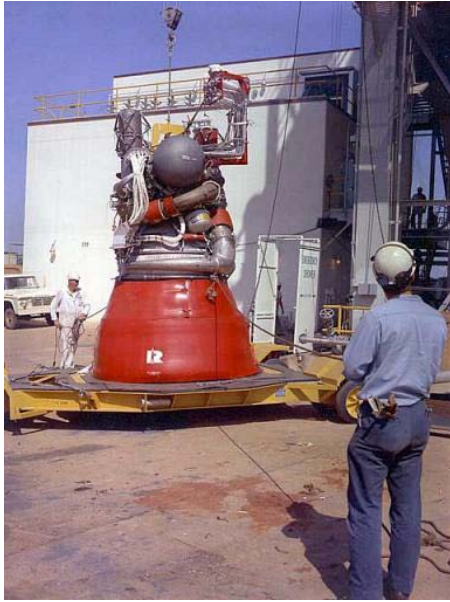
Figure 24. J-2 Engine being Hoisted to the J-4 Test Capsule
