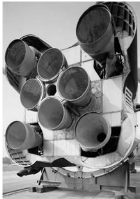
Figure 6. Saturn SA-1 Vehicle Model in the NASA/Lewis 8 X 6 – Ft Wind Tunnel
