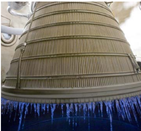
Figure 41. CECE Deep Throttling Engine being Tested in PWR's E-6 Facility
