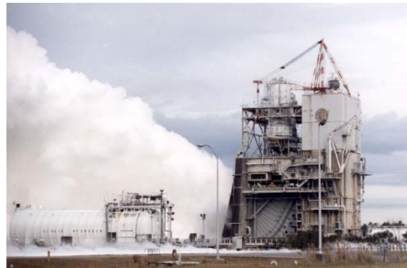
Figure 43. SSME Firing at the Stennis Test Stand A2
