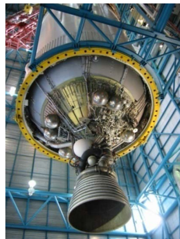
Figure 20. Douglas S-IVB Stage and Rocketdyne J-2 Engine
