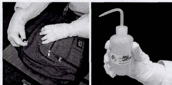
Fig. 3. Robonaut A being teleoperated in the handling of the zippers and Velcro on a backpack, and handling a squeeze bottle for dispensing liquids
