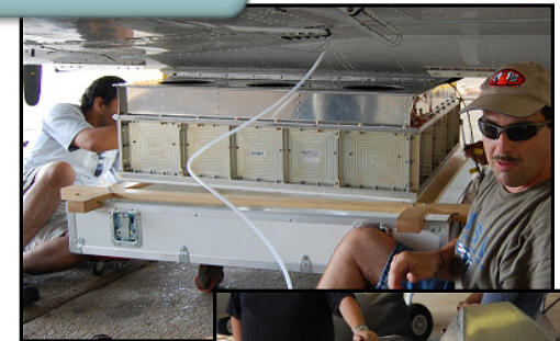
Adapter box provides interface between antenna and aircraft
