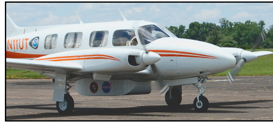
Belly pod fairings fabricated in-house at UTSI
