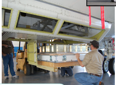
Structural interface for antenna inside bomb bay
