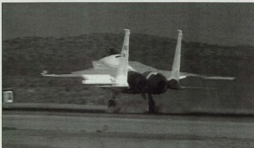
Figure 2. This Airplane Landed under PCA-system control only; no other flight controls were used.
