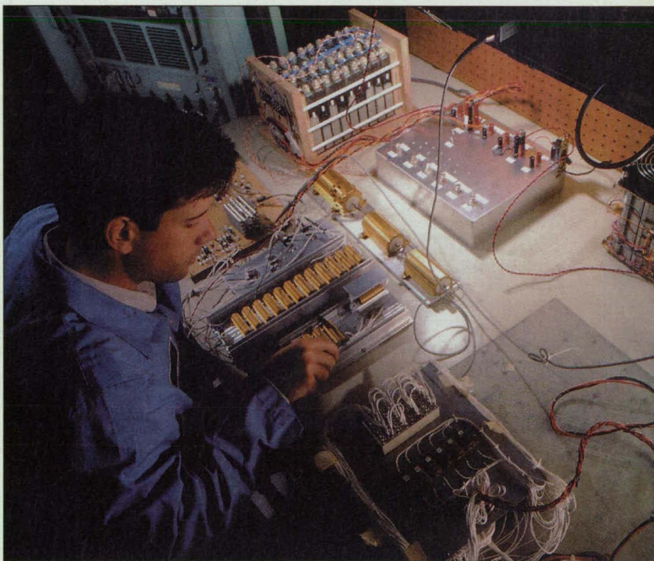
Spacecraft-designed options and operational scenarios are quickly assessed on the Mars Pathfinder Power Subsystem Breadboard at JPL.
