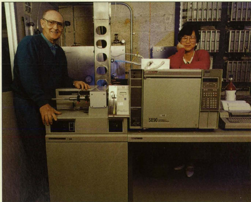
Shown with NASA Lewis's gas chromatograph mass spectrometer (GCMS), which identifies and precisely measures the concentration of molecular species in a gas sample to parts per billion, are Ted Brabbs (NYMA) and Dr. Chowen Wey (OIA), who developed the measurement technique.
