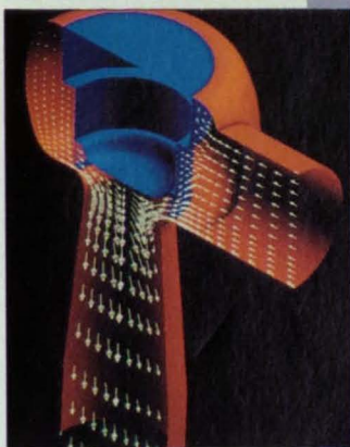
Velocity vectors reveal flow patterns through the center section of this steam turbine inlet throttle valve.
