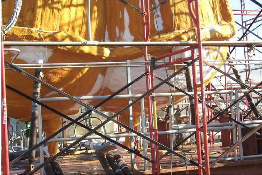
Figure 61: Ice formation and thermal performance loss on the X33 tank SOFI insulation by mechanical breakage, weathering, cracking and moisture penetration.
