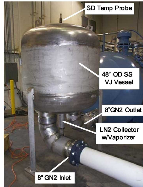
Figure 17. The GN2 phase separator final assembly.
