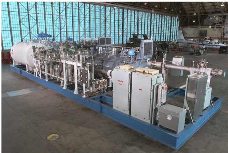
Figure 2. The Liquid Oxygen Propellant Densification Unit (PDU) in the final stages of check-out and assembly at the NASA GRC Hangar.
