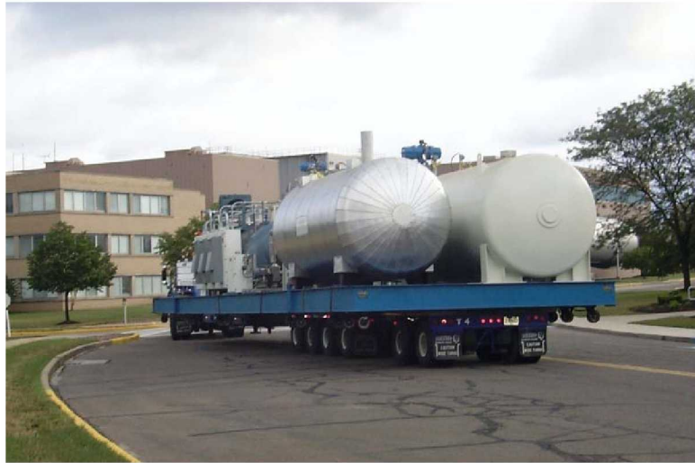
Figure 19. The LO2 densifier is self-contained and modular for ease of transportability as illustrated by this move at the NASA GRC in 1999.
