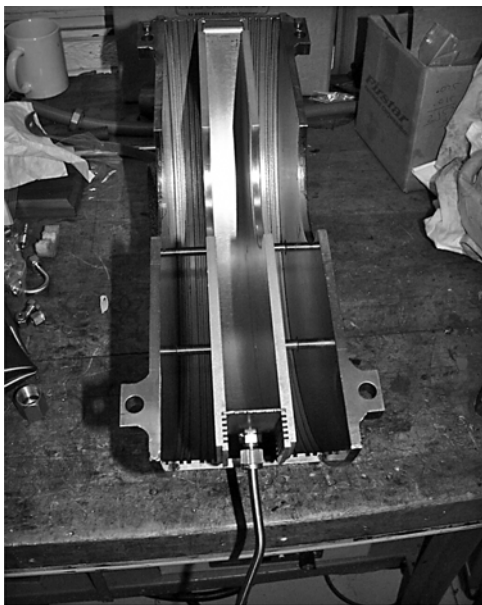
Fig. 4: Shroud before installation in test facility, showing adjustability of clearance radially and axially.
