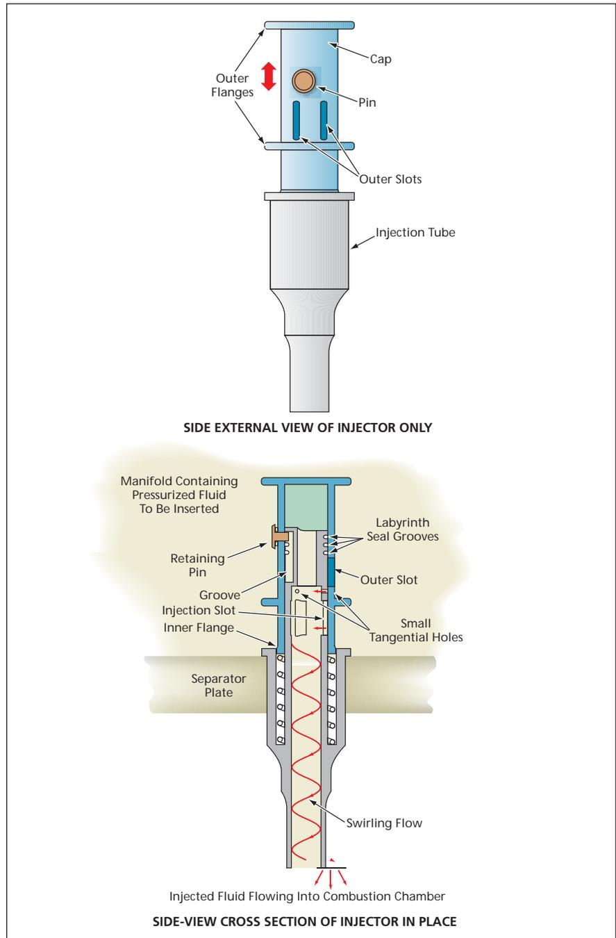
The Cap Would Slide in the Injector Tube in response to a change in pressure drop from the manifold above the separator plate to the combustion chamber below the injector outlet. The sliding would expose more or less of the injector-slot area to adjust the pressure drop according to the flow rate. This configuration is representative, not exclusive: the basic self-adjusting-injector concept could be implemented by a variety of mechanisms.
