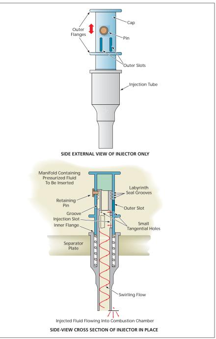
The Cap Would Slide in the Injector Tube in response to a change in pressure drop from the manifold above the separator plate to the combustion chamber below the injector outlet. The sliding would expose more or less of the injector-slot area to adjust the pressure drop according to the flow rate. This configuration is representative, not exclusive: the basic self-adjusting-injector concept could be implemented by a variety of mechanisms.
