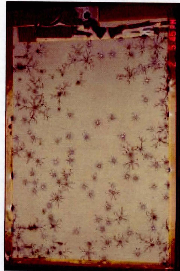
Anodized Al Plate After Repeated Arcing
