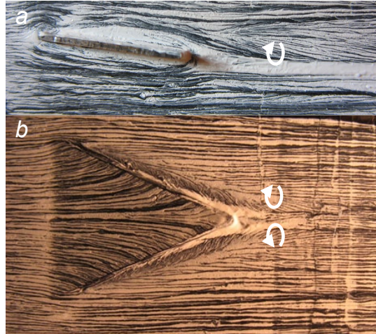
Figure 10.—(a) Surface oil-flow visualization of the streamwise single-sign and (b) vortex pair formation.
