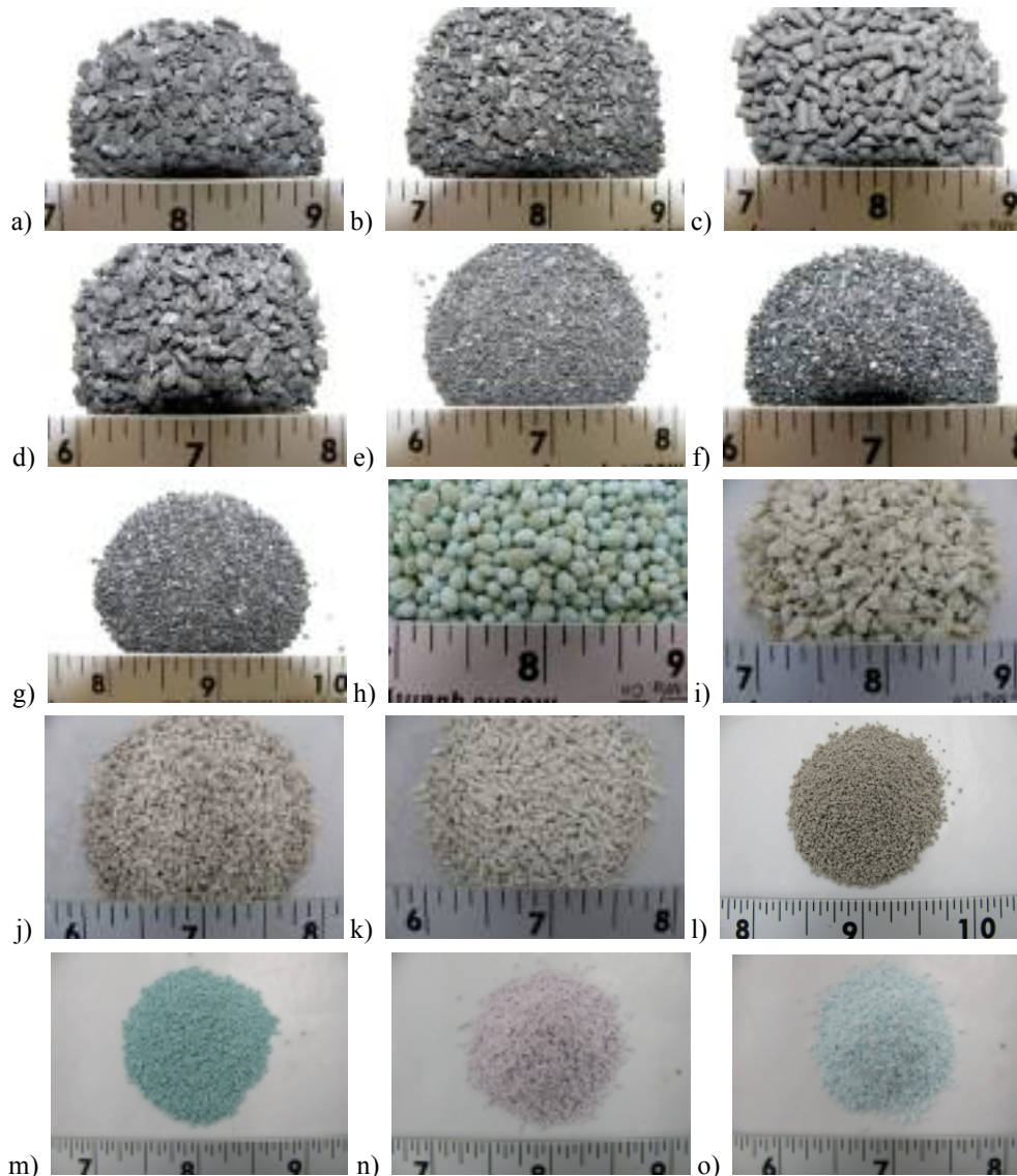
Figure 1. Materials evaluated to date for NH 3 removal capacity. a) B-S Type 3032 carbon, b) Calgon Carbon Ammonasorb II, the vendor's 'replacement' carbon, c) Nucon International Ammosorb I-3, d) Tigg HP, e) 3M 6004 amine/methylamine mask cartridge, f) Molecular Products Chemsorb 1425, g) Dräger Dragercarb, h) Modern Safety Techniques LTCAT, i) Tigg KLS zeolite, j) St. Cloud natural zeolite, k) UOP HISIV 3000. l) Co-X zeolite m) Cu-X zeolite n) Co-Y zeolite o) Cu-Y zeolite. Scale markers in inches.
