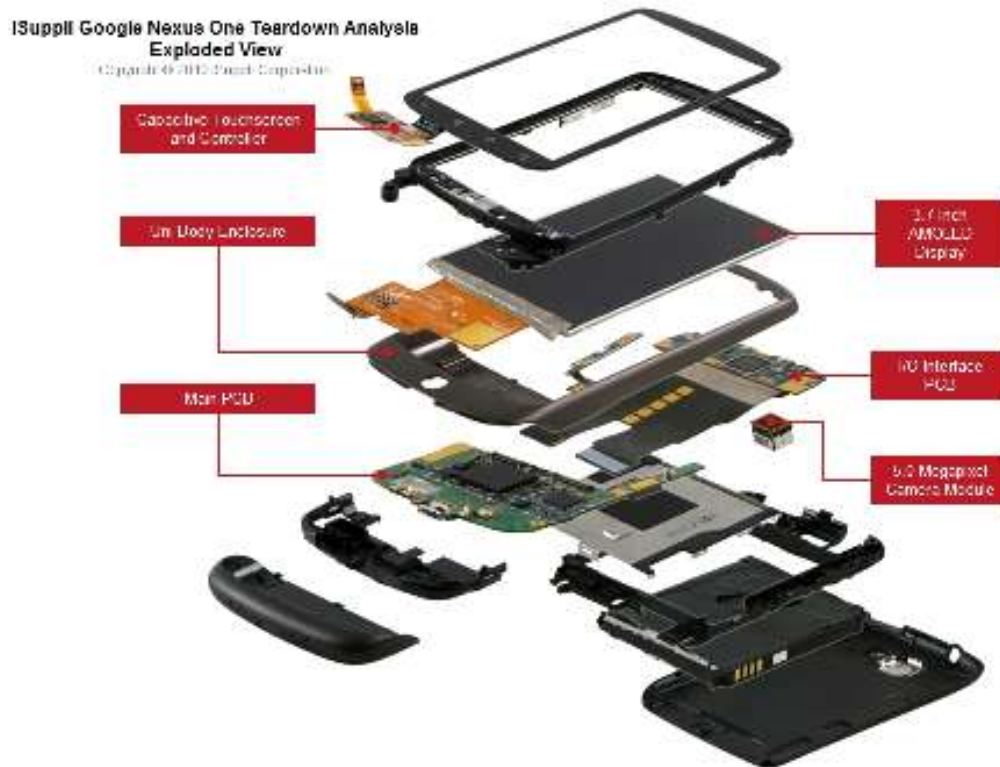
Figure 3 Exploded view of the Nexus One. Source: (Rassweiler, 2010)
