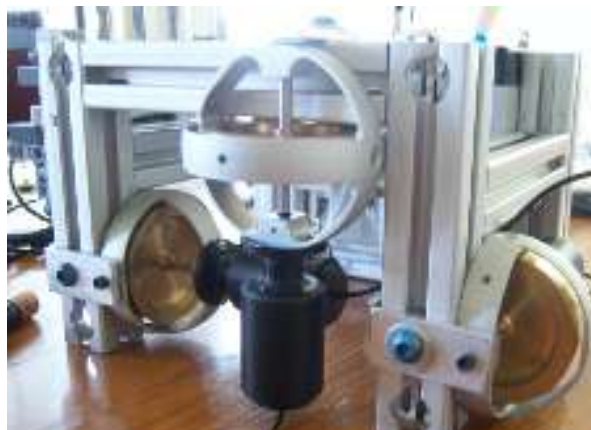
Figure 5 Gyroscopes accommodated in the Phonesat
