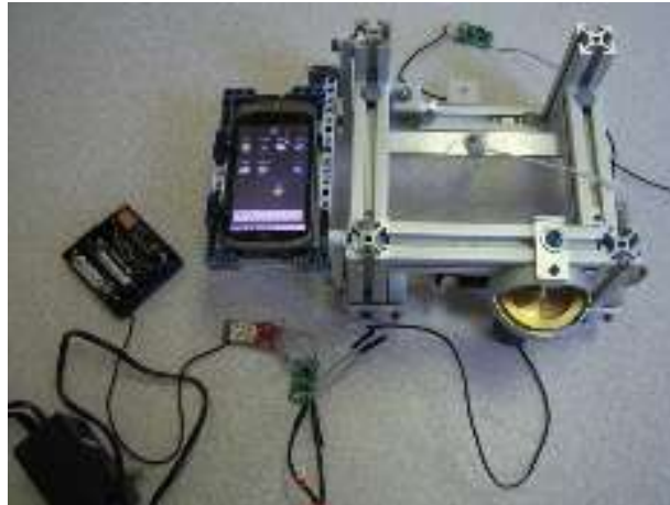
Figure 4 PhoneSat in its first structure model
