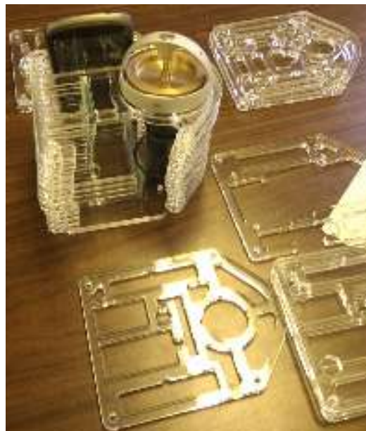
Figure 13 Structure for test a gyroscope and two cell phones
