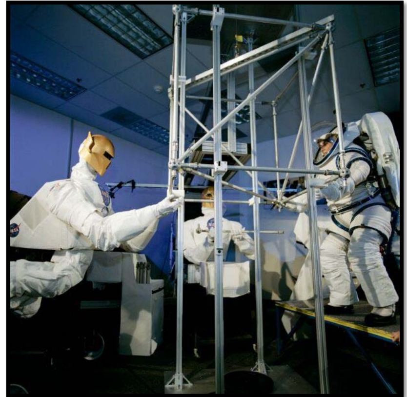
Astronaut Nancy Currie works with 2 Robonauts to build a truss structure during an experiment.
