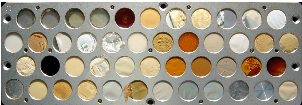
Figure 3. Post-flight photograph of the MISSE 2 PEACE Polymers experiment.
