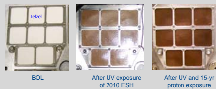
Figure 3. Test Phase 1 Coupon Configuration (ETFE samples pre and post UV and LEP exposures)
