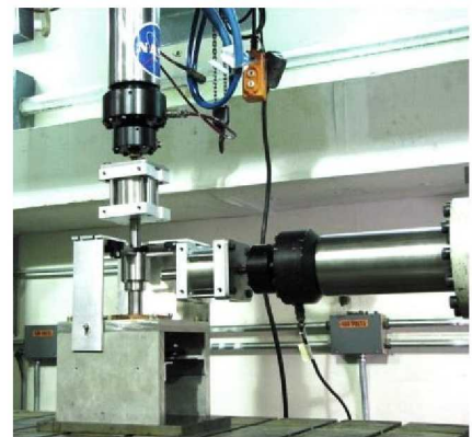
Figure 3. Servo-valve-controlled hydraulic actuators in the Instron in-plane biaxial load frame. The actuators were used to apply external loads to the test article.
