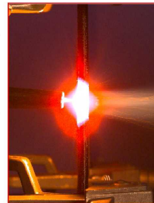
Thermal barrier for Shuttle and Atlas V SRM nozzle joints
