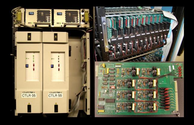
The WDPF system contained OCR-161 controllers and large Q-line I/O cards.
