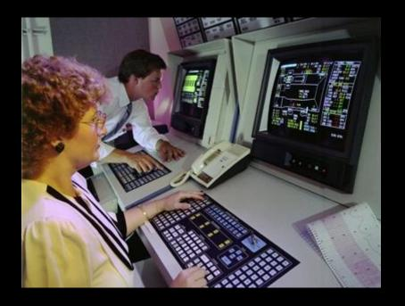
The WDPF systems included state-of-the-art 8 color graphics on WEStation operator consoles with bulky CRT monitors and chiclet keyboards.
