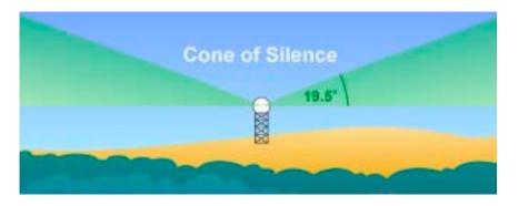
Figure 1. Cone of Silence for WSR-88D 'NEXRAD' radar systems
