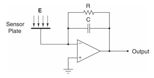
Figure A1-2. Simplified sketch of the preamplifier circuit in an electric-field sensor.
