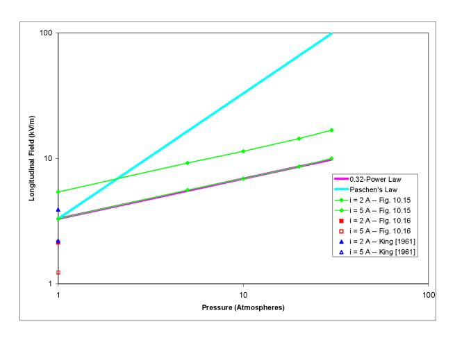
Figure A5.4. Experimental Data on Arc Potential Gradient vs. Pressure
