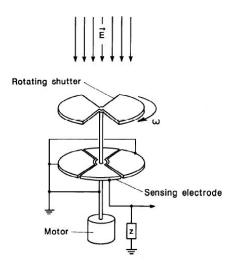
Figure A1-1. Sketch of an electric field mill (from IEEE Standard 1227)
