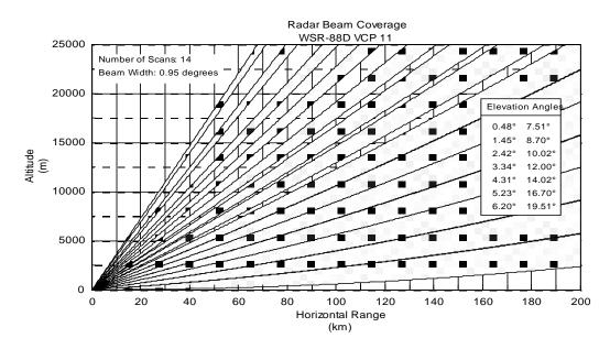
Figure A9.1. Radar beam coverage for 'Volume Coverage Pattern 11' of the WSR-88D radar
