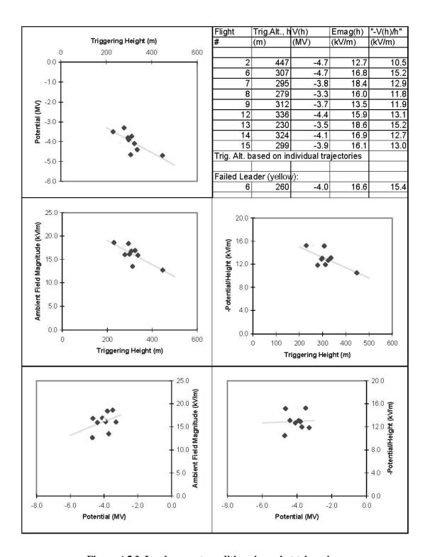
Figure A5.3. Leader-onset conditions in rocket triggering
