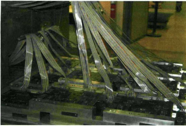
Figure 6 Test Vehicles in the HALT/HASS Chamber
