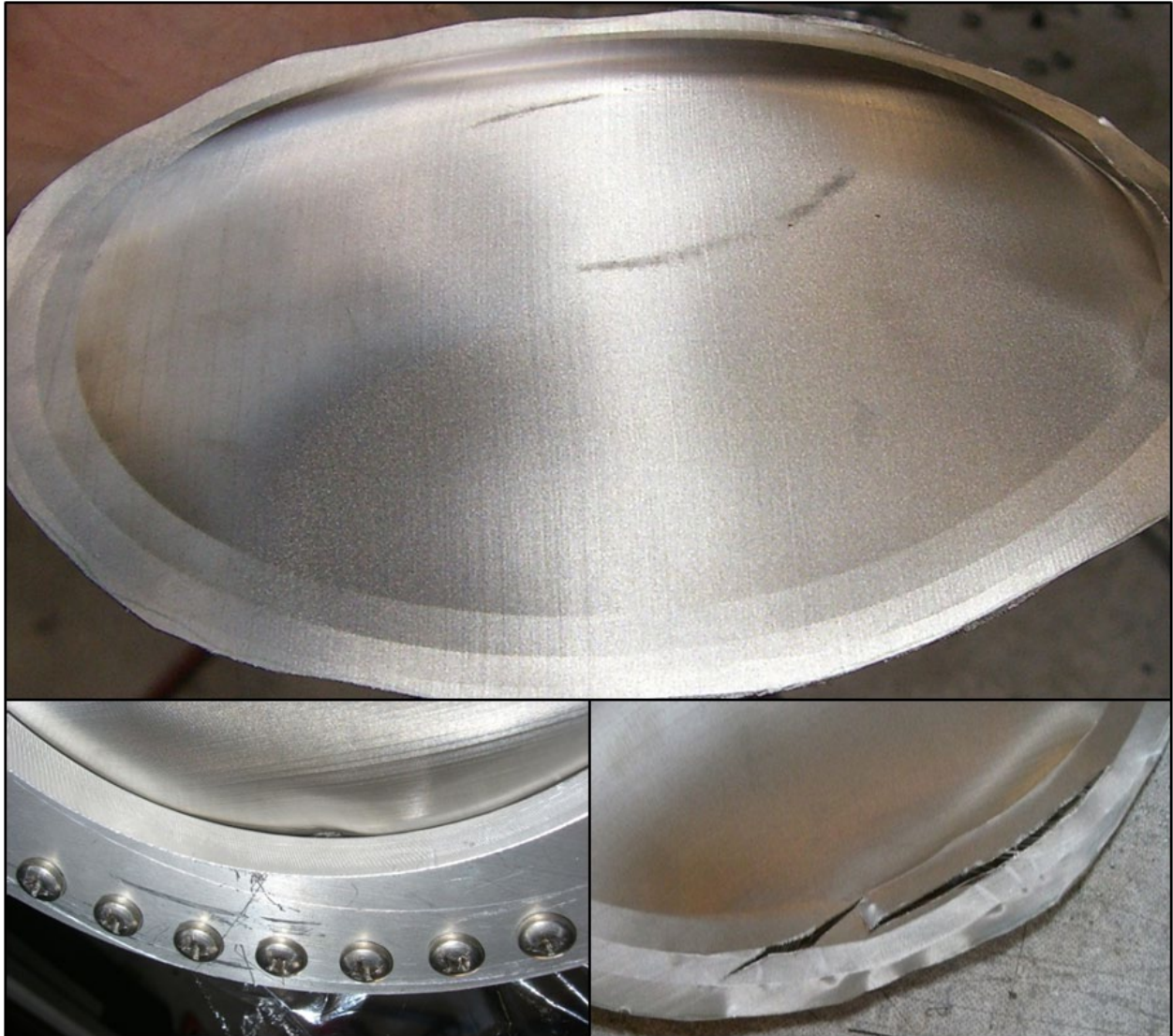
Figure 45.—Images of yielded screen to retain spherical contour (top) and over yielding of screen (bottom-left) and yielding to tear (bottom-right).
