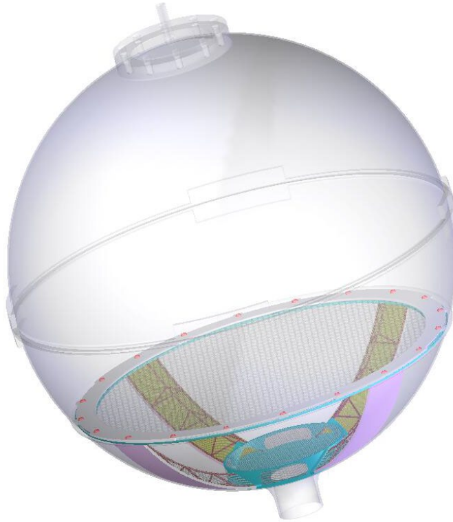
Figure 6.—Descent stage RCS partial PMD/four-channel gallery.
