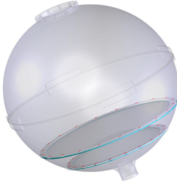
Figure 35.—Concept No. 2—Descent stage RCS tank dual flexible screen design.
