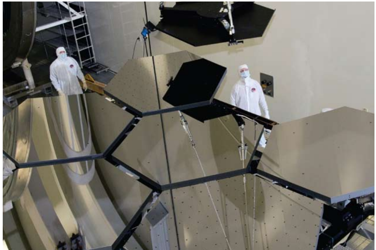
The primary mirror for the James Webb Space Telescope will have 18 hexagonal-shaped mirror segments, each measuring 1.3 meters in diameter. Here, the mirror segments are being prepped to move into the X-ray and Cryogenic Facility at NASA's Marshall Space Flight Center.
