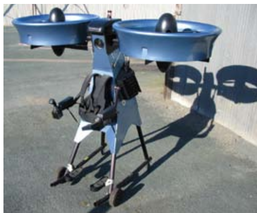
Trek Aerospace's Springtail EFV is a single operator powered-lift vehicle that supports the operator/pilot in a standing position.
