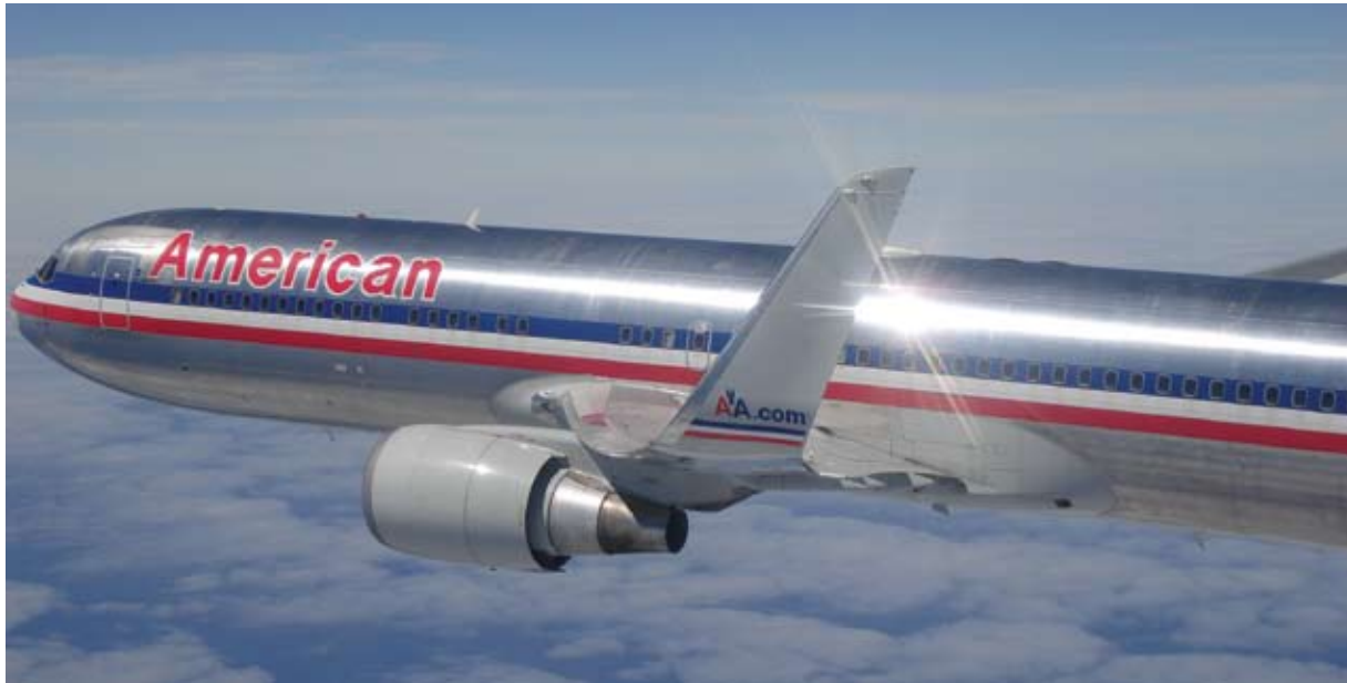
Aviation Partners Boeing manufactures and retrofits Blended Winglets for commercial airliners. The technology typically produces a 4- to 6-percent fuel savings, which can translate to thousands of gallons of fuel saved per plane, per year.
