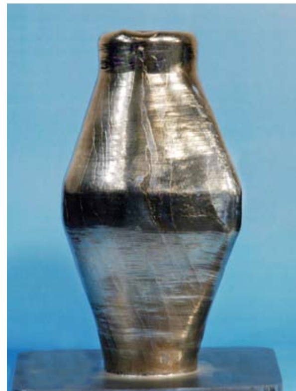
This structural metal part was fabricated from EBF3, an advancement in layered part fabrication.
