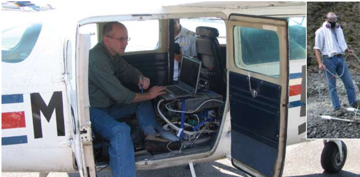
Tim Griffin works with the mobile leak detector before a sampling flight. The shuttle leak detection system used at the launch pads is the size of three refrigerators, but Griffin's team reduced it in size and added automation so it could be mobile.
