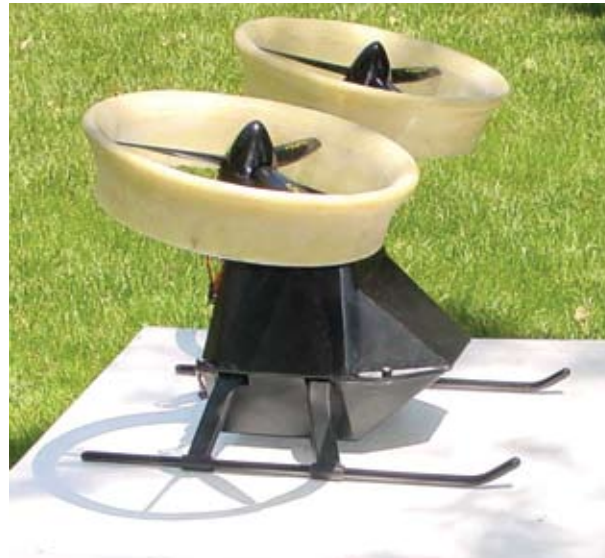
The OVIWUN, a miniaturized version of Trek Aerospace Inc.'s larger, manned vehicles, allows researchers to test designs and experiment in a smaller, safer, more contained setting.
