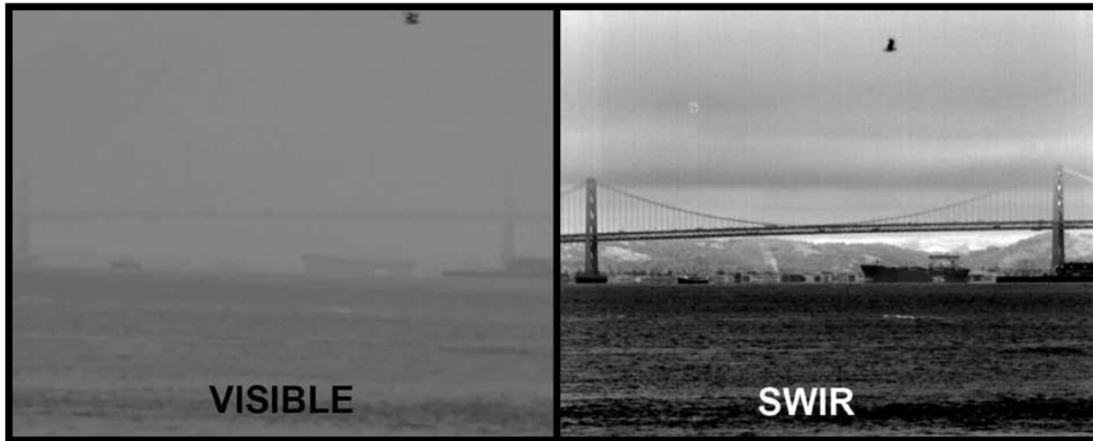
These images of San Francisco Bay show the difference between images produced by a visible light camera and a SWIR camera. The visible light image (left) shows mostly fog; the SWIR image (right) reveals detail through the fog. SWIR technology detects reflected light at wavelengths that the human eye cannot see, in bands on the electromagnetic spectrum between the visible and thermal.
