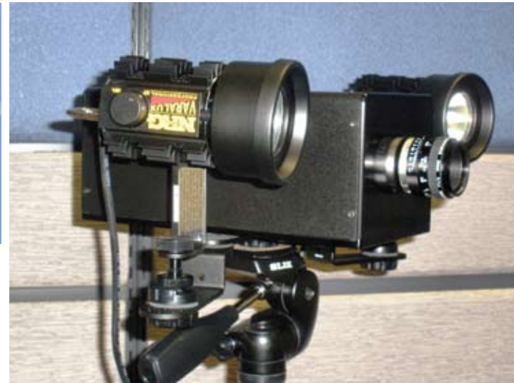
Based on the hyperspectral imaging sensors used in Earth observation satellites, NASA engineers and Institute for Technology Development researchers collaborated on a portable design for imaging the health of farmers' crops. Exclusively licensed by Themis Vision Systems LLC, the company has developed compact, 4-pound systems that can fit on multiple platforms (right). One medical application for the technology is imaging for skin cancer, cervical cancer, and breast cancer surgery. The images above show cancer on a patient's nose.
