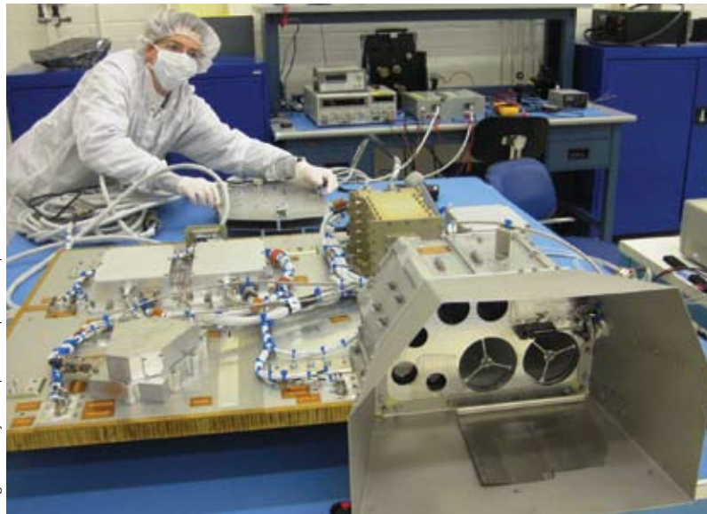
The science payload panel (left) for LCROSS (in the artist rendering above) underwent final testing at Ames Research Center in late 2007. The Data Handling Unit built by Ecliptic Enterprises Corporation is the gold box near the center.
