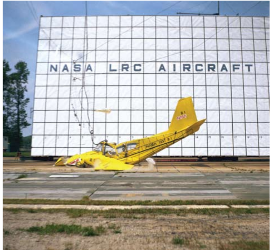
Originally built to allow Apollo astronauts to practice landing on the Moon, this 240-foot-high gantry (left) is now Langley Research Center's Landing and Impact Research Facility. Crashworthiness testing at the facility (right) allowed Cirrus Design Corporation to improve survivability during stall/spin impacts.
