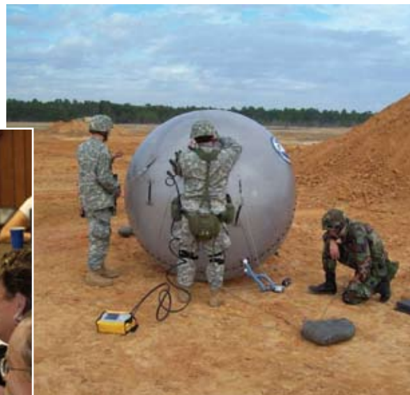
The inflatable antenna can provide backup communication (left) when land lines are down. In the aftermath of Hurricane Ike, GATR Technologies volunteered the use of the antenna to provide high-bandwidth communications for local residents. Soldiers (above) deploy and test an inflatable antenna at Fort Bragg, North Carolina.
