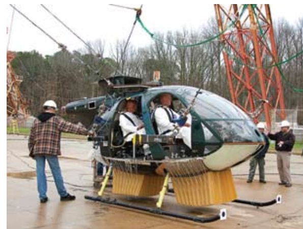
Researchers at Langley are testing the deployable energy absorber with the help of a helicopter donated by the Army, a crash test dummy contributed by the Applied Physics Laboratory in Laurel, Maryland, and a 240-foot-tall structure once used to teach astronauts how to land on the Moon.
