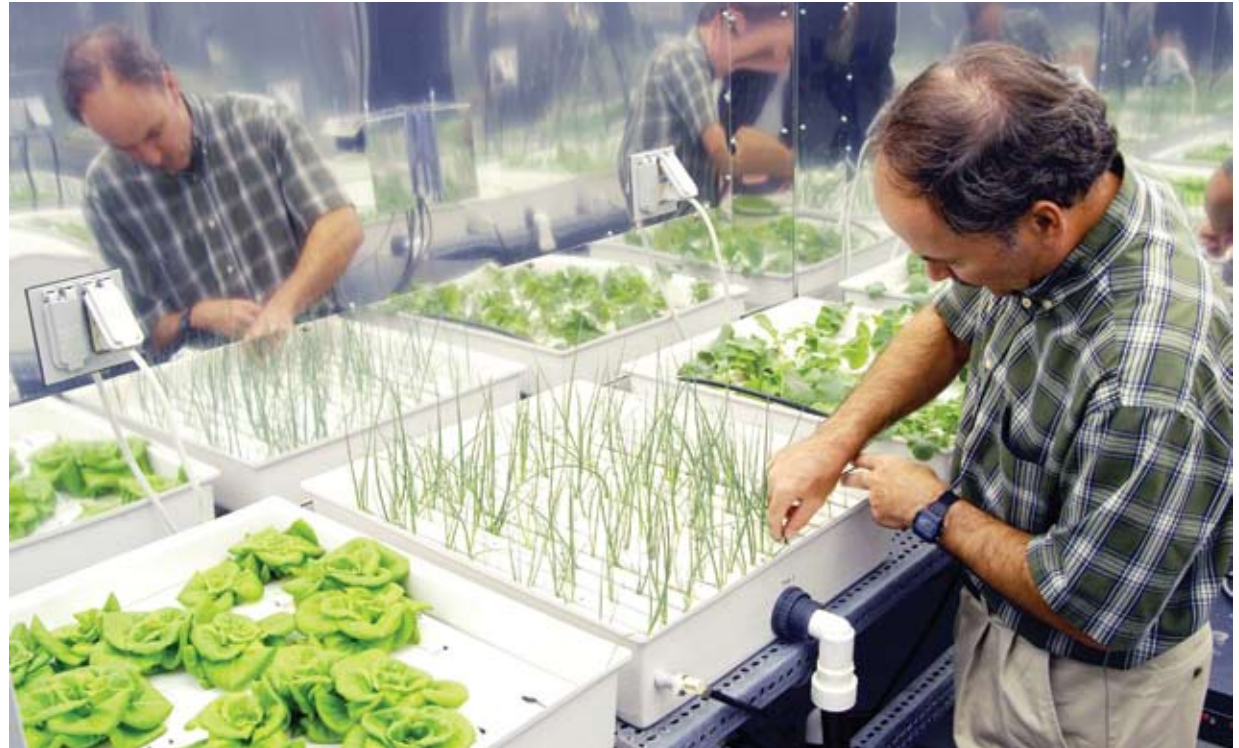
Hydroponic techniques—like those used to grow these onions, lettuce, and radishes in this plant growth chamber in Kennedy Space Center's Space Life Sciences Laboratory—may one day contribute to the development of a bioregenerative life support system.
