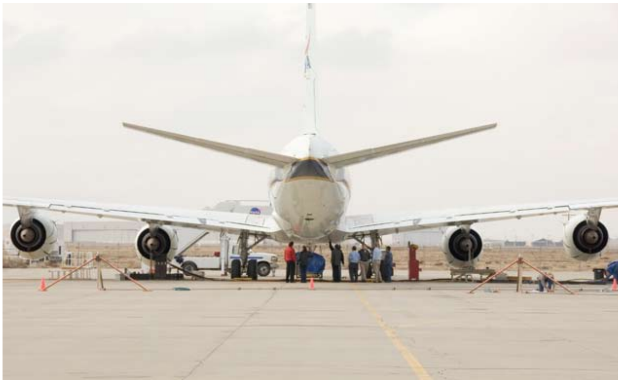
Test instrumentation is set up behind the inboard engines of NASA's DC-8 airborne science laboratory during alternative fuels emissions and performance testing at NASA's Dryden Aircraft Operations Facility in Palmdale, California.
