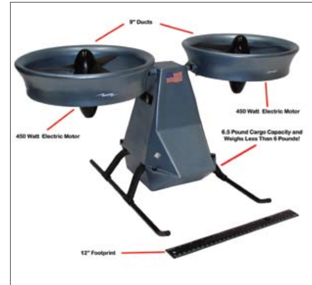
The OVIWUN, a miniaturized version of Trek Aerospace Inc.'s larger, manned vehicles, allows researchers to test designs and experiment in a smaller, safer, more contained setting.
