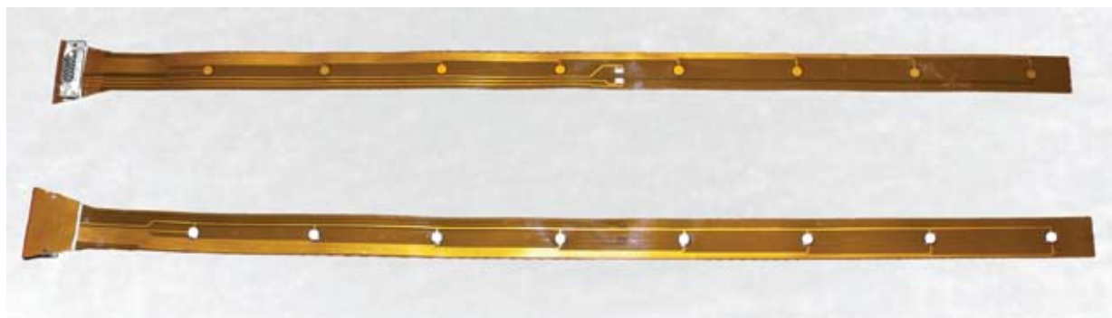
Acellent’s SMART Layers can be customized with two or more sensors in a strip unit, like the eight-sensor strips shown here, to monitor structural health conditions such as strain and moisture.
