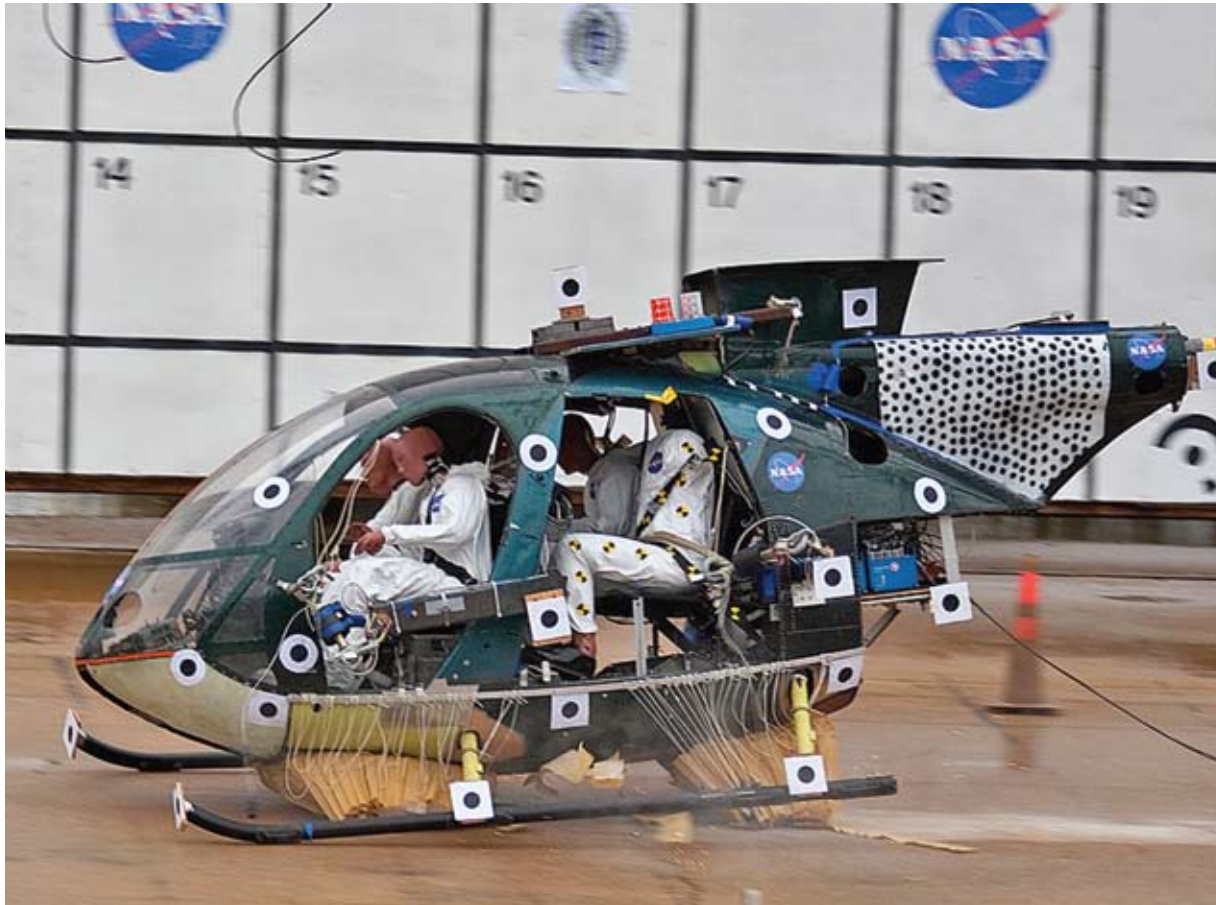
A honeycomb-type airbag that was created to cushion astronauts may end up in helicopters to help prevent injuries.
