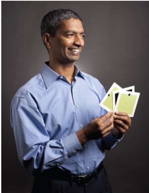
Each of Bloom Energy's fuel cells, such as those held by company CEO K.R. Sridhar above, can produce 25 watts—enough to power a light bulb. The cells can be stacked to increase the power output. The lime-green coating is the anode side; the black coating is the cathode side.
