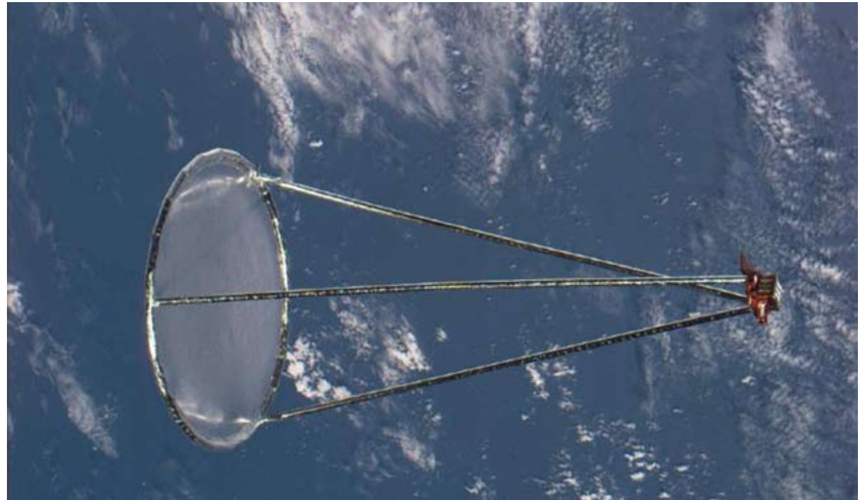
The Inflatable Antenna Experiment, seen here fully deployed from its Spartan satellite, logged its data on an SBIR-derived solid-state recorder (SSR) developed by SEAKR Engineering Inc.
