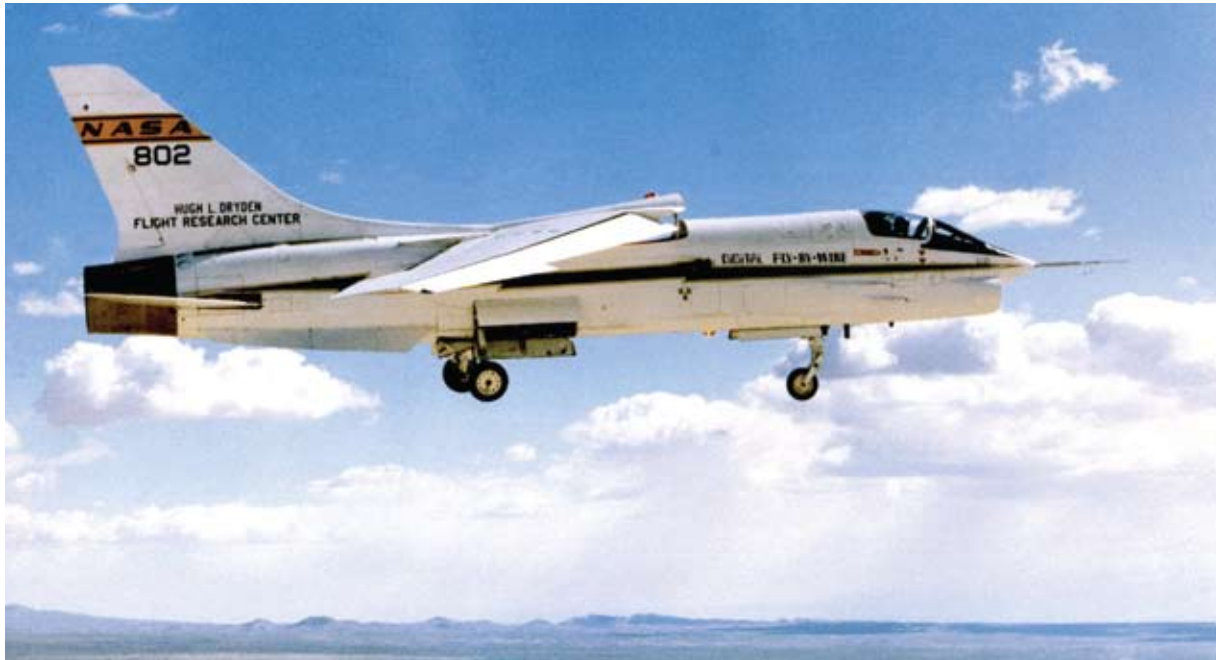
This modified F-8 Digital Fly-By-Wire Crusader was the test bed of the fly-by-wire flight control systems now used on the space shuttles and military and civil aircraft to make them safer, more maneuverable, and more efficient. Digital fly-by-wire and its developers were inducted into the Space Technology Hall of Fame this year.
