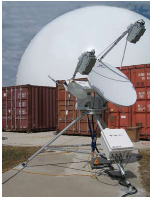
The NASA Narrow-beam Multi-waveband Scanning Radiometer (NNMSR), seen here with the CHILL radar in the background, can determine possible icing conditions along a flight path.
