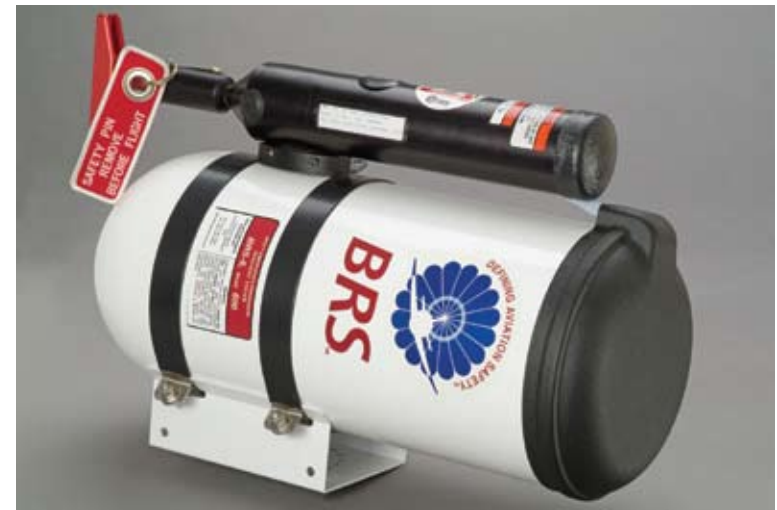
This BRS Aerospace Inc. parachute system, designed for sport aircraft, deploys its chute (contained in the white canister) in less than 1 second, thanks to a solid rocket motor (the black tube on top).
