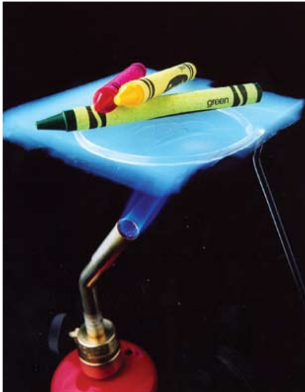
Crayons placed on top of a piece of silica aerogel will not melt from the heat of a flame. Certain types of aerogel provide 39 times more insulation than fiberglass.
