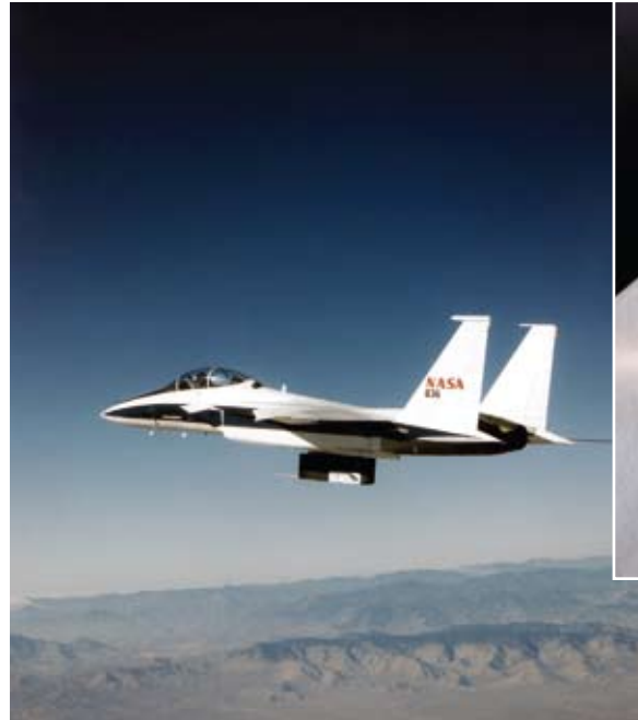
Dryden Flight Research Center's F-15B test bed aircraft flew several flights to determine the location of sonic shockwave development as air passes over an airfoil. The shock location sensor (above), developed by Tao of Systems Integration Inc., isolated the location of the shock wave to within a half-inch.
