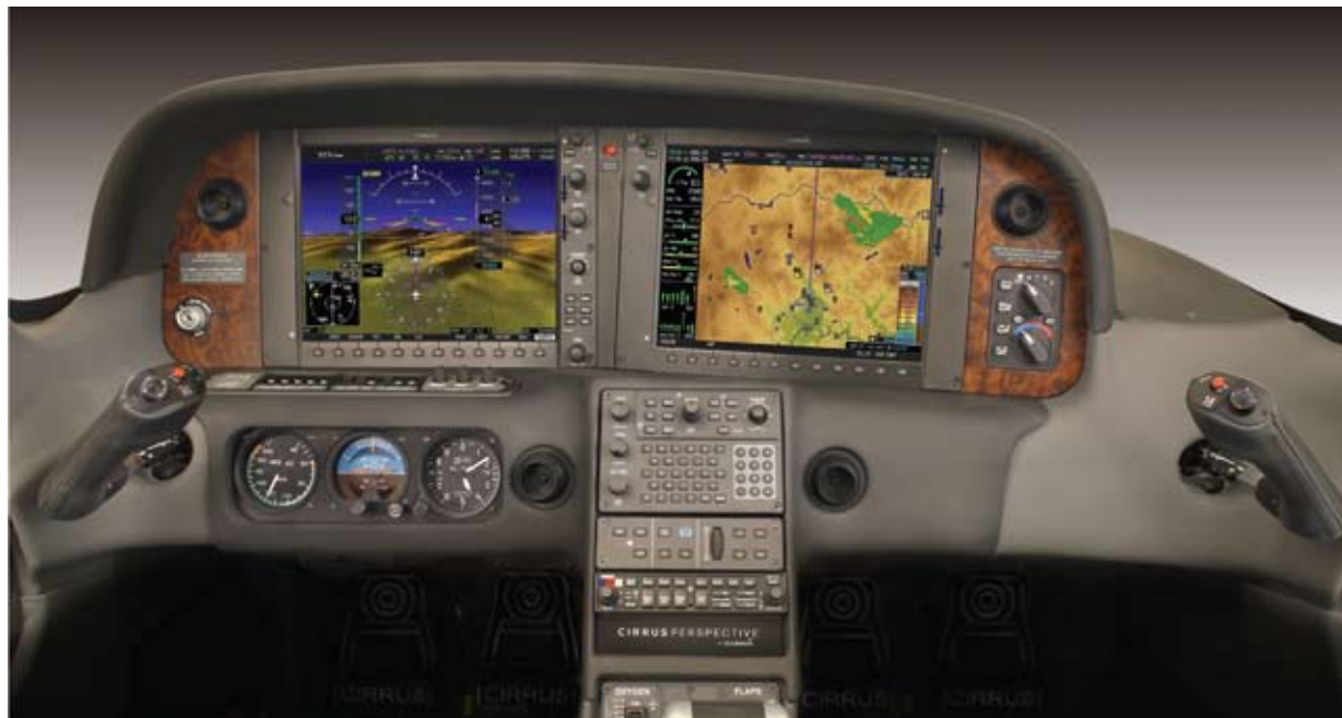
Cirrus' synthetic vision systems trace their roots to innovations in glass cockpit technology developed under the NASA-led Advanced General Aviation Transport Experiments consortium.
