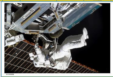
STS111-E-5238 (11 June 2002) --- Perrin/MS1 (France) installs the Mobile Remote Servicer Base System (MBS) on the ISS
