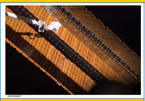
ISS016-E-009207 (3 Nov. 2007) --- While anchored to a foot restraint on the end of the OBSS, Parazynski/EV1 assesses his repair work as the solar array is fully deployed during EVA 4.
