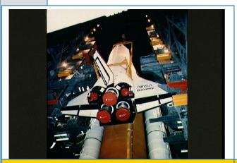
ABOVE: S89-28089 & KSC-89PC-26---OV-103, suspended by overhead crane hooked to support structure attached at four points, is lowered for mating to ET & SRBs at KSC VAB Bay 1. SSMEs are covered with protective red shields BELOW: STS029-04-029---CDR Coats on OV-103's forward flight deck
