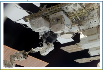
S118-E-06998 - Anchored to the foot restraint on the Canadarm2, Williams, and Mastracchio (out of frame), R&R a faulty control moment gyroscope (CMG-3) into the Z1 truss during EVA 2.
