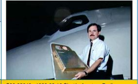
S90-32048 1990-03-16 Shuttle Amateur Radio Experiment (SAREX) equipment held by R. Parise/PS at the JSC Full Fuselage Trainer. SAREX is used to conduct shortwave radio transmissions between ground amateur radio operators and a licensed onboard operator (in this case, Parise).
