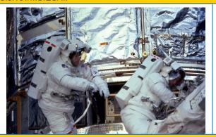
STS103-731-051 (19-21 December 1999) --- Foale (left) and Nicollier/ESA (on end of RMS) replacing one of HST's Fine Guidance Sensors (FGS).
