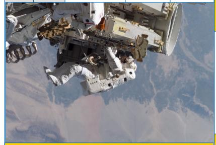
S115-E-05623 (12 Sept. 2006) --- Piper, releases the restraints on the forward Solar Array Blanket Box (SABB) during EVA with Tanner, partially visible at top edge of frame.
