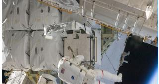
S132-E-008106 -- Bowen during first EVA with Reisman (out of frame), continues construction and maintenance on the ISS, with battery replacements & installation of a 2nd Ku-band antenna.
