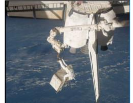
S135-E-007515 --- With his feet secured on a restraint on the ISS robotic arm or Canadarm2, Ron Garan/ Exp 28 Flight Engineer, carries the pump module,
