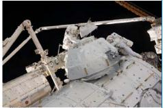
ISS022-E-067184 --- Behnken (left) & Patrick removing insulation blankets & launch bolts from Cupola's windows.
