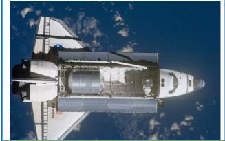
ISS028-E-015565 Atlantis as seen from ISS brings supplies & spare parts to ISS packed in MPLM at rear of P/L Bay. Last flight of the "Banana Truck"! [Atlantis was happily called the "Banana Truck" on STS-71 by Cosmonaut Strehalov, see page 2-84.]
