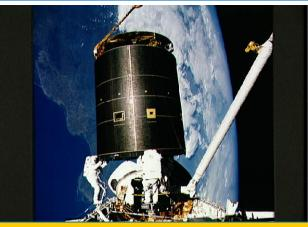
STS049-91-020 1992-05-16 STS-49 crewmembers complete successful capture of the International Telecommunications Organization Satellite (INTELSAT VI) during EVA3. Left to right, Hieb/MS, Akers/MS, & Thuot/MS, on RMS, have handholds on the satellite and prepare to attach capture bar (tethered to Hieb). Two earlier grapple attempts on two-person EVA's were unsuccessful.
