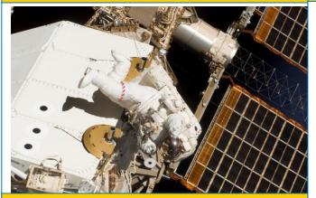
S123-E-006089 --- Reisman, Exp 16 & Linnehan (out-of frame) prepare tool change out mechanisms on Dextre during EVA 1.
