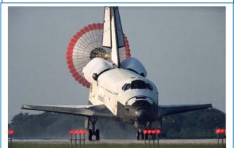
STS050-S-106 - First flight of OV-102 with drag chute, INWS, etc. (Second flight of drag chute - deployed after NLGTD).
