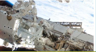
S123-E-006729 --- Linnehan (right) & Behnken install a spare-parts platform and tool-handling assembly for Dextre during EVA 3.
