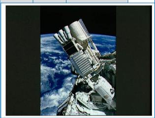
s35-13-008 -- Wisconsin Ultaviolet photo-Polarrimeter Experiment (WUPPE) on Spacelab pallet. The Broad Band X-Ray Telescope (BBXRT) is behind this pallet and is not visible.
