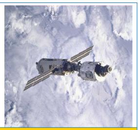
STS088-703-032 --- Blanketing clouds form the backdrop for the connected Zarya and Unity modules after release from Endeavour's cargo
