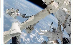
STS112-326-033 --- Wolf (left) & Sellers during 2nd EVA. Wolf is anchored to a foot restraint on ISS's Canadarm2 while Sellers traverses along the airlock spur.
