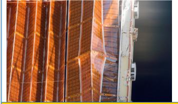
S116-E-05789 - A kink occurred in the port-side P6 solar array during the first attempt to retract that array on Dec. 13, 2006.
