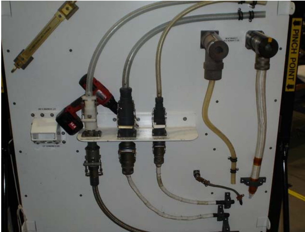
Figure 2. Busy board included handrail removal/installation and several quick-disconnect stations.
