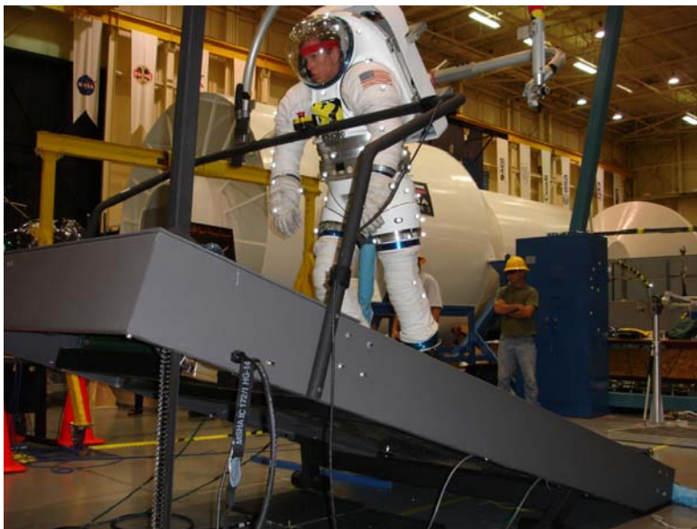
Figure 5. Suited subject performs inclined treadmill locomotion.
