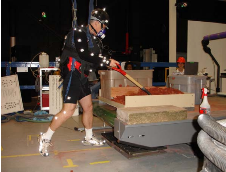
Figure 4. Instrumented unsuited subject wearing an X-Vest and performing shoveling task (metabolic emphasis).
