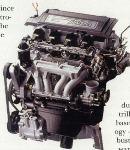
Honda's Civic Hybrid features a gasoline-electric powertrain with a battery pack that recharges automatically.
