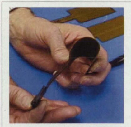
A Flex Patch Is Very Flexible , even though it contains a piezoceramic wafer that, taken by itself, would be extremely brittle and could not be bent as much as shown here.
