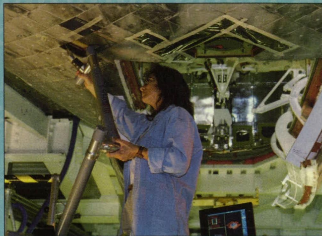
The arm probe measures every irregularity in the tile cavity, including screw and rivet heads in the body of the vehicle. The arm can measure objects to a dimensional tolerance of \pm 0.003 inches.
