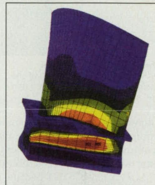
This CARES/LIFE plot shows stress levels on a turbine blade.
