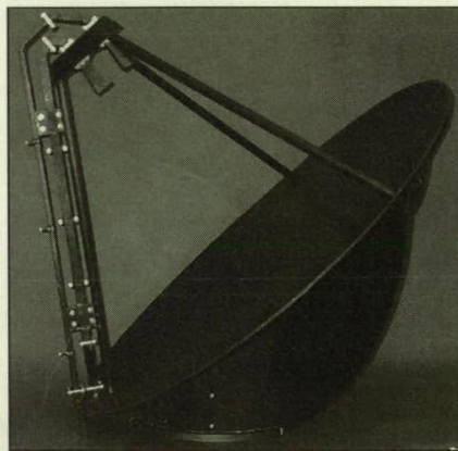
This Dual-Beam Reflector Antenna features a lightweight composite-material structure. The aperture is elliptical, with major and minor axes of 1.07 and 0.96 m, respectively. The total mass is only 6.4 kg.
