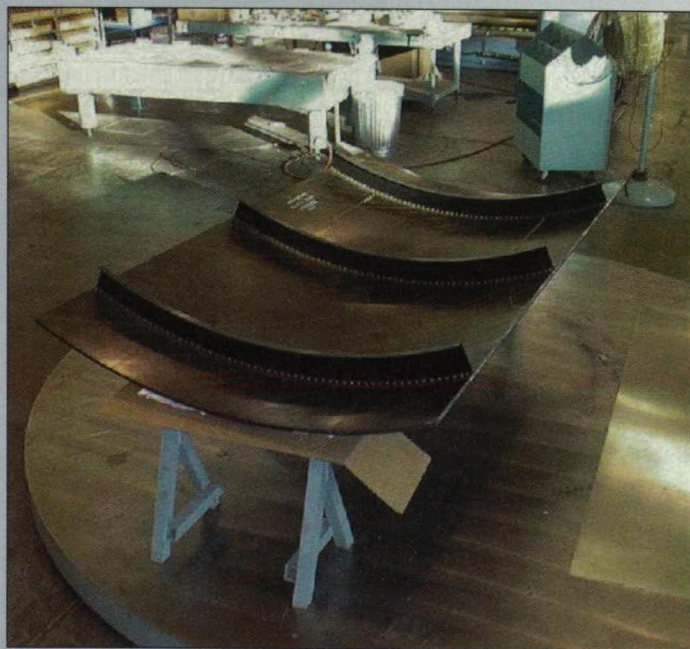
PETI-5, a versatile, high-temperature resin and adhesive, was used in the fabrication of this fuselage subcomponent. The material also cures into a tough, heat-resistant plastic that is easily formed into complex parts.
