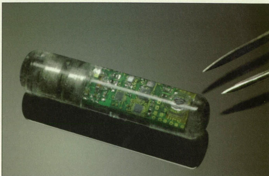
Figure 2. A Prototype Transmitting Unit would be miniaturized and encapsulated in biocompatible silicone rubber.
