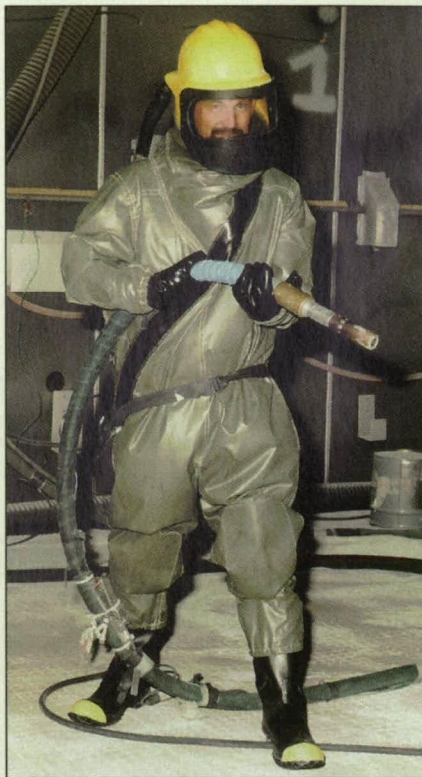
The ECAB Protects the Worker from the hazards of abrasive blasting, and offers advantages over older, multiple-garment protective ensembles.
