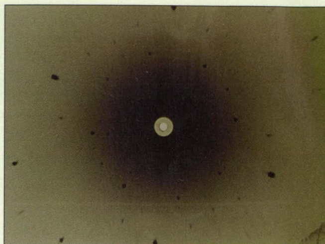
Figure 2. A Back-Reflection Laue X-Ray Diffraction Pattern from the pre-form in Figure 1 confirms its single-crystal nature.
