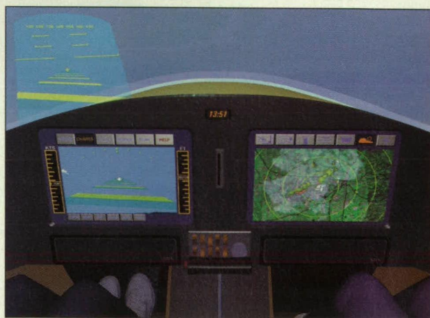
This image depicts the single-engine aircraft instrument panel showing computer-generated displays.
