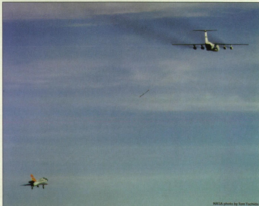
Figure 2. The C-141A Airplane Towed the QF-106A Airplane in flight tests. The airplanes were connected by a tow rope 1,000 ft (305 m) long.
