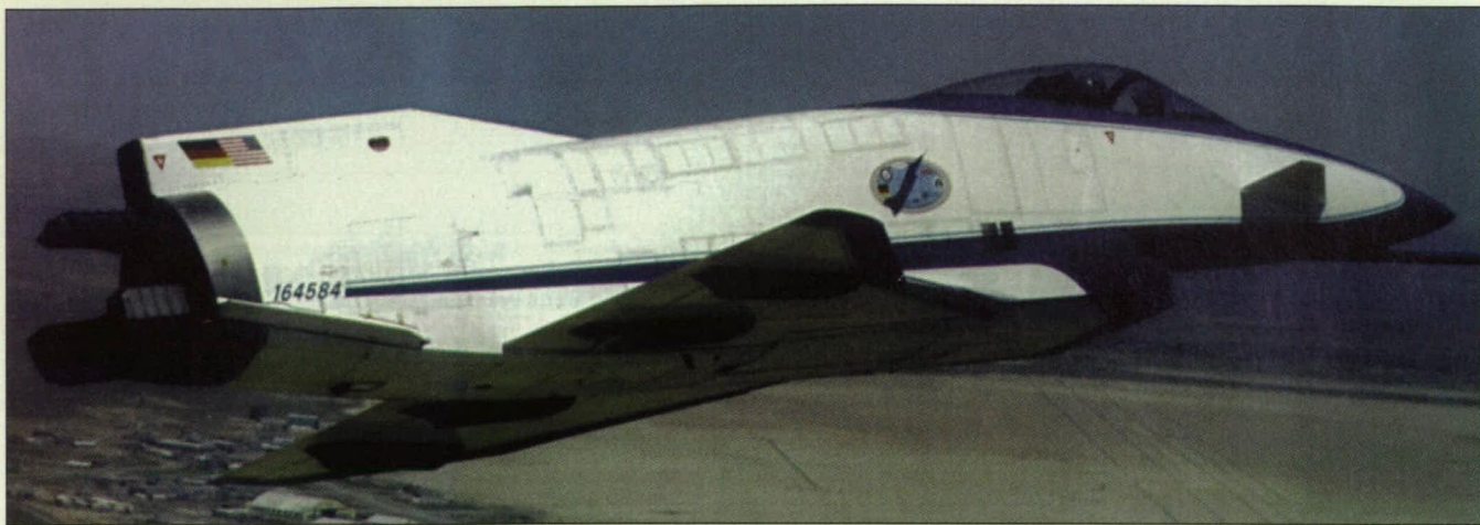
The X-31A Airplane was operated with thrust vectoring in a quasi-tailless mode to test and demonstrate advanced control concepts.
