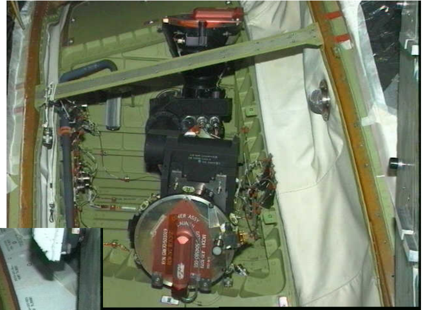
Thermal Blankets Removed
