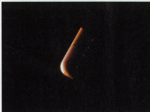
Assembled Interlocking Tiles (Modular Design) During Successful Test in Arc Jet at Surface Temperature Near 2,400 °F
