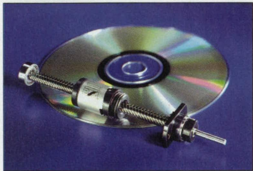
Self-lubricating polymers give lead screw assemblies the ability to operate in clean environments. Their simplified mechanism (compared with ball screws) makes them cost-effective while advances in materials allow more aggressive operation than previously possible. This has made them popular in such industries as medical and semiconductor.
