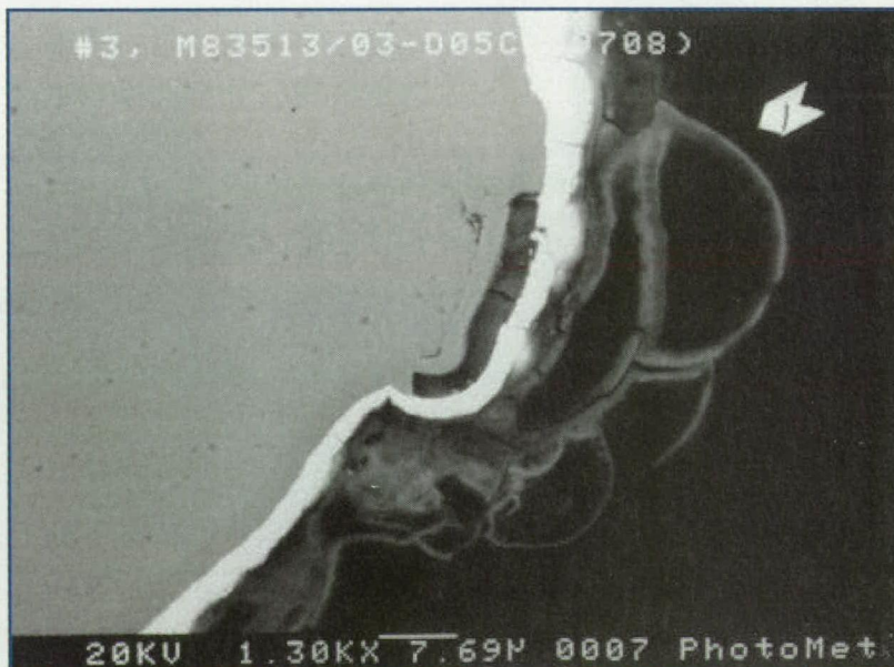
A closeup of the cross section of corrosion salts on a gold-plated nickel-underplated copper contact. The fluorine had attacked, reduced, and removed nickel from under the gold, creating a nickel-fluoride salt on the contact surface.
